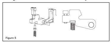
To install, first lubricate the trigger and disconnect pin bores with the supplied ALG Go-Juice. Pre-assemble the disconnect and trigger using the slave pin. Insert the trigger assembly into the lower receiver while making sure the trigger spring legs rest against the bottom of the receiver well and extend forward from the trigger.
